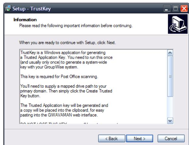
The Trustkey application will create a trusted application key for GWAVA 4.5 to access the Post Office with administrator rights. The information dialog also details exactly what is required to create the trusted application key.
