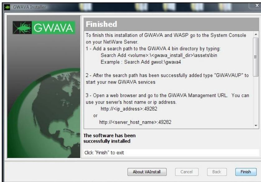
NetWare: Follow the onscreen instructions to add a search path and start GWAVA. GWAVA 4 has now been successfully installed. Click 'Finish' and continue with the installation process by following the instructions in the server activation section.
