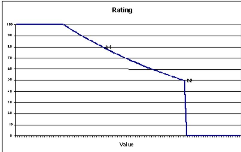
The formula that is used to interpolate the rating curve is an exponential curve through the two points  $(b_1, R_1)$  and  $(b_2, R_2)$ :
