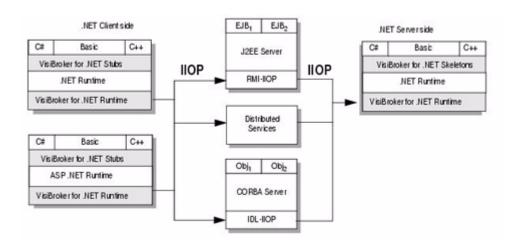
Figure 1.1 VisiBroker for .NET client-side deployment diagram
