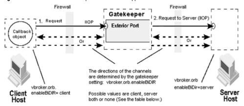
In the figure above, GateKeeper sits between the client and server and therefore it acts as a server for the client and as a client for the server. The Client/GateKeeper and the GateKeeper/Server communication channels can be set to unidirectional or bidirectional connections.
