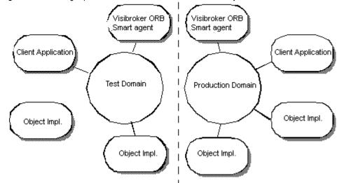
VisiBroker allows you to distinguish between multiple VisiBroker ORB domains on the same network by using unique UDP port numbers for the Smart Agents of each domain. By default, the OSAGENT\_PORT variable is set to 14000. If you wish to use a different port number, check with your system administrator to determine what port numbers are available.
