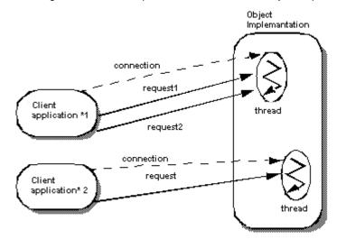
Client application #1. The same thread that handles request 1 will handle request 2. The thread blocks request 2 until it completes request 1. (With thread-per-session, requests from the same Client are not handled in parallel.) When request 1 has completed, the thread can handle request 2 from Client application #1. Multiple requests may come in from Client application #1. They are handled in the order that they come in; no additional threads are assigned to Client application #1.
