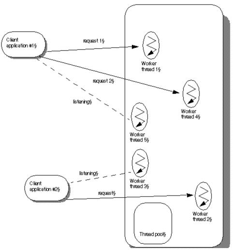
The above figure shows that when a second request comes in from Client application #1, it uses worker thread #4. Worker thread #5 is spawned to listen for new requests. If more requests came in from Client application #1, more threads would be assigned to handle them, each spawned after the listening thread receives a request. As worker threads complete their tasks, they are returned to the pool and become available to handle requests from any client.
