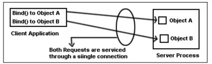
The following figure shows the connections for a client using multiple threads that has several threads bound to an object on the server.
