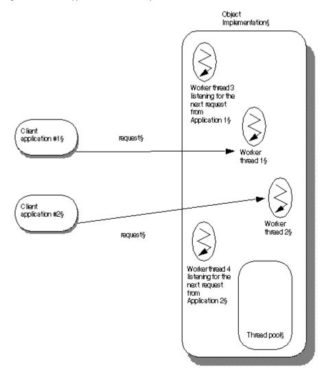
As the above figure shows, when Client application #2 establishes its own connection and sends a request, a second worker thread is created. Worker thread #3 is now listening for incoming requests.
