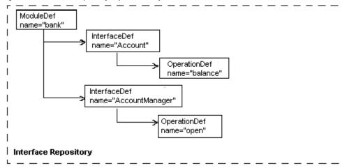
The OperationDef object contains references to additional data structures (not interfaces) that hold the parameters and return type.
