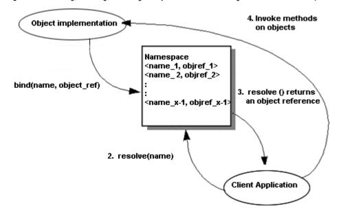
Figure 15.1 Binding, resolving, and using an object name from a naming context within a namespace
