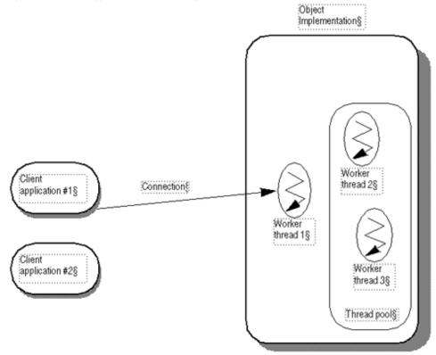
In the above figure, Client application #1 establishes a connection to the Object Implementation and a thread is created to handle requests. In the thread pool, there is one connection per client and one thread per connection. When a request comes in, a worker thread receives the request; that worker thread is no longer in the pool.
