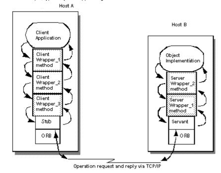
Figure 25.4 Multiple, typed object wrappers registered
