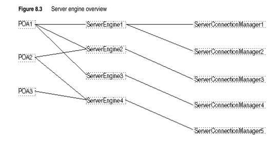
The simplest case is where POAs have their own unique single server engine. Here, requests for different POAs arrive on different ports. A POA can also have multiple server engines. In this scenario, a single POA supports requests coming from multiple input ports.
