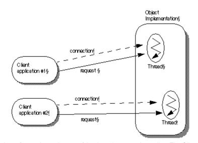
The above figure shows the use of the thread-per-session policy. The Client application #1 establishes a connection with the object implementation. A separate connection exists between Client application #2 and the object implementation. When a request comes in to the object implementation from Client application #1, a worker thread handles the request. When a request from Client application #2 comes in, a different worker thread is assigned to handle this request.
