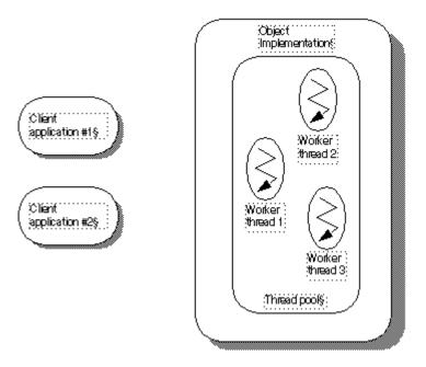
The figure above shows the object implementation using the thread pool policy. As the name implies, there is an available pool of worker threads in this policy.
