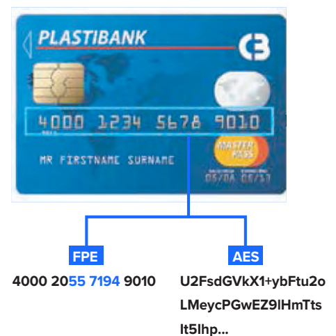
Figure 2. Voltage Format Preserving Encryption
