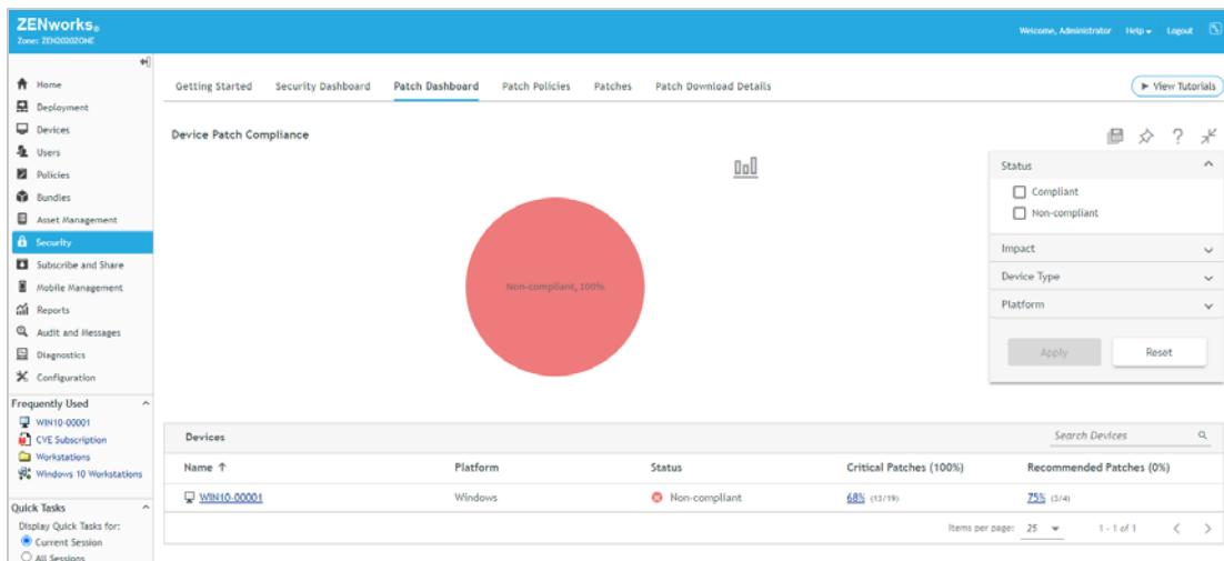
In the example above, the Windows 10 device is listed with a status of *Non-compliant*. By default, compliance requires 100% of all applicable Critical (security) patches to be installed and the device has only 64% (13/19) installed. The default compliance does not require any Recommended patches to be installed, which means that the default compliance is determined strictly from Critical patches.
