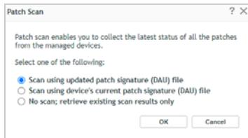
4 Keep the default selection (**Scan using updated patch signature (DAU) file**) so that the recently created DAU file will be distributed to the device before the scan, then click **OK** to display the Quick Task Status dialog.
