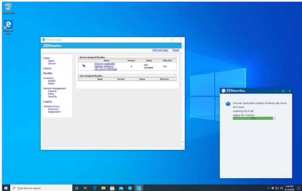
Once the scan completes, the View Progress dialog is cleared and the status of the DAU bundle changes from Not Installed to Available.
