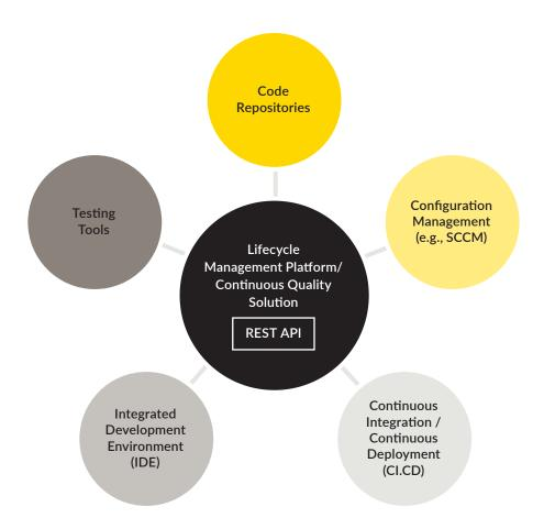
Figure 2 – Typical integrations required for continuous quality.
